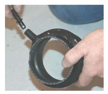
Slide 90-110 mm clamps on either side of the hump hose and then slide the hump hose onto the MAF housing. Rotate the hump hose such that the nipple will locate just above the throttle body motor (roughly 10 o'clock position, see pictures). Rotate the MAF sensor assembly such that the logo on the sensor housing is at the top and lines up with the logo on the air-bridge.
