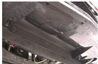
To remove the radiator shroud you need to temporarily disconnect and remove the engine oil cooler.
