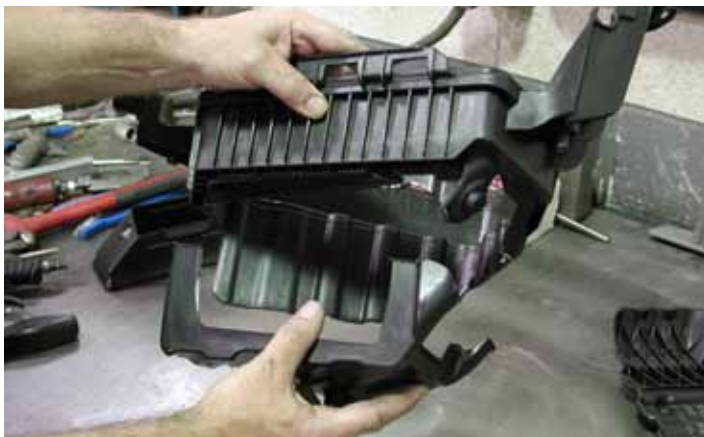
20. Cut the airbox along your marked lines. After the final cuts have been made, your new airbox should look like this.
