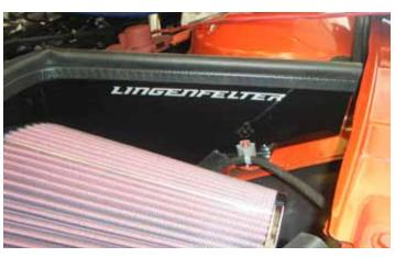
26. If desired, install the Lingenfelter decal onto the interior of the airbox by peeling the paper off of the back of the decal, pressing the decal onto the airbox, and finally peeling the front piece of paper off of the decal.
