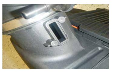
8. Using a 7mm socket, remove the two (2) screws that secure the MAF sensor to the airbox. Make sure to keep the stock MAF sensor as it will be re-used for the new air intake installation. Take care not to drop or otherwise damage the MAF sensor.
