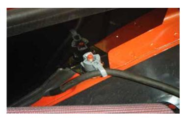
25. Tighten the airbox flange nut and then attach the retaining clip back onto the upper stud as well.
