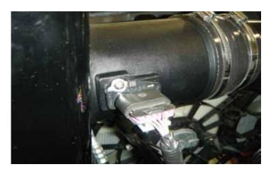
21. Connect the MAF sensor harness connector to the MAF sensor. You should hear a click when the connector is fully engaged. Slide the grey tab to lock the MAF sensor connector in place.
