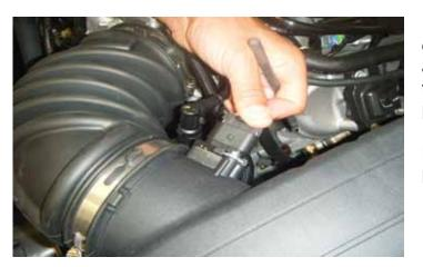
3. Unplug the Mass Air Flow (MAF) sensor connector, which is located on the side of the airbox inlet, by first sliding the grey tab to unlock the connector. Then, press on the center tab and pull the connector away from the airbox inlet.
