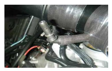
18. Insert the supplied 45 degree breather hose adapter into the supplied throttle body hump hose. Clock the adapter so that it points straight up, as shown in the picture.
