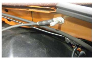
22. Using a 10mm socket, remove the ground stud located on the front driver-side corner of the engine compartment.
