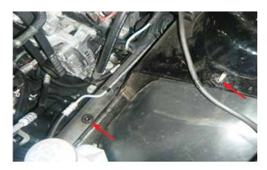
13. The arrows in the adjacent image show the two (2) mounting locations for the airbox.
