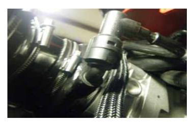
20. Connect the stock PCV tube to the 45 degree breather adapter.
