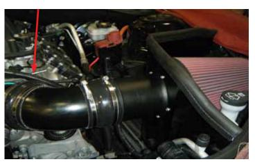
19. Rotate the inlet elbow clockwise until it can be connected to the throttle body. Connect the hump hose to the throttle body. Disengage all four (4) of the worm gear clamps and place the clamps over the narrow parts of the hump hoses. Using an 7mm socket, secure the hump hoses. Do not overtighten. To improve the appearance you may want to align all of the clamps in the same direction and position.
