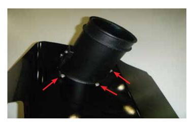
9. Insert the supplied MAF housing into the hole in the supplied airbox. The MAF housing should be clocked as shown in the image to the left. Using a Phillips head screwdriver and the five (5) supplied 10-32 screws, secure the MAF housing to the airbox. The screws should be tightened in a star pattern.
