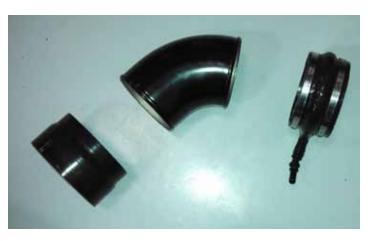
16. The air inlet duct work includes a hump hose with vent tube, metal duct and an adapter hose. The metal duct is directional with the longer straight section pointing towards air box assembly. The adapter hose should be installed on the end between the air box assembly and duct with the larger diameter end going over the MAF housing. The hump hose should be connected between the metal duct and the throttle body. See image to the left for clarification.
