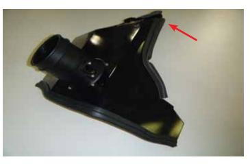
12. Firmly push the supplied shorter edge seal with the angle cut on one end onto the bottom of the airbox. The angle cut in the edge seal should be pointed down when the airbox gets installed into the vehicle, as shown by the arrow.
