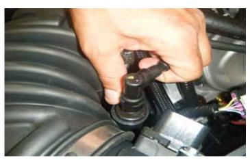
6. The positive crankcase ventilation (PCV) tube goes from the driver-side valve cover to the rubber air inlet tube. Disconnect the PCV tube from the air inlet tube by pressing the retaining tab on the fitting and pulling up on the tube.
