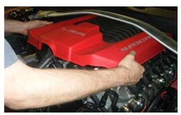
2. Remove the engine cover by pulling the front of the cover up and away from the engine.
