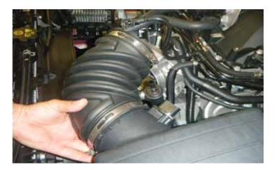
7. Remove the air inlet tube from the throttle body and pull up on the airbox to remove the air inlet tube and airbox assembly.
