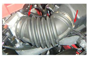
4. Loosen the hose clamps securing the rubber air inlet tube to the throttle body using an 8mm socket.
