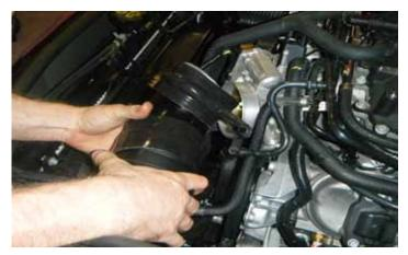
17. Install the hump hose and the adapter hose onto the metal inlet duct. To make installation easier, connect the inlet elbow to the MAF sensor housing and point the other end of the elbow upward, as shown in the picture. If necessary, silicone lubricant can be applied to the inside of the silicone hoses to make the assembly easier to adjust.
