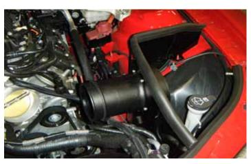
14. Lower the airbox assembly onto the bottom grommet and the upper stud as shown in the image to the left. Firmly push down on the airbox to verify that the airbox is fully seated onto the grommet.
