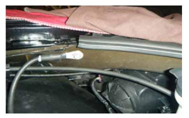
23. Using a 10mm socket, install the supplied ground bolt (PN 11588712). Torque the bolt to 89 in-lbs.
