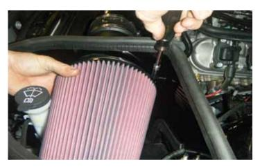
24. Carefully install the supplied air filter onto the MAF housing inside the airbox. If the airbox flange nut was left loosened, you can move the airbox slightly towards the passenger side of the vehicle to make installation of the air filter easier. Secure the air filter to the MAF housing using the large supplied worm gear clamp and an 8mm socket. Do not overtighten.
