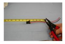
9) Strip the ends of the new fuel pump harness wires.
