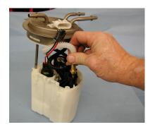
25) Connect the fuel pump harness connector to the top of the module.
