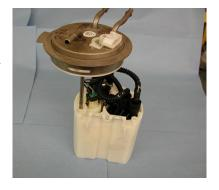
2) Unplug all the wires from the bulkhead connector at the top of the module.
