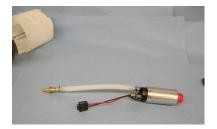
15) Slide the supplied foam fuel pump sleeve over the end of the pump. Position the sleeve at the top of the pump.
