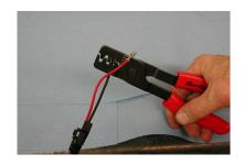
11) Assemble the new fuel pump wires into the connector that was removed from the old fuel pump wires. The black wire going into terminal A and the red wire goes into terminal B.
