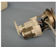
20) Lightly lubricate the O-ring on the bottomn of the fuel pressure regulator.
