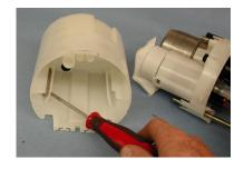
23) Slide the bucket onto the bottom of the module, making sure the regulator slides into the passage in the bucket. Make sure the bucket is fully seated onto the module and the regulator is seated into the bucket.
