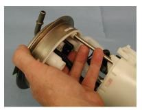
26) Follow the GM service instructions for installing the fuel pump module back into the vehicle. Use the supplied replacement fuel pump module O-ring.
