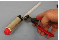
13) Slide the other Oetiker clamp over the other end of the fuel hose. Install the supplied fuel filter adapter fitting into the end of the hose. Crimp the clamp into position over the adapter fitting.
