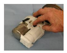
21) Clock the pump so that the sock can fold up inside the bucket.
