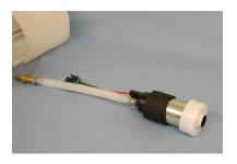
17) Install the supplied fuel pump prefilter (filter sock) over onto the inlet of the pump. Gently press the pump into the filter sock against a clean work bench until fully seated.
