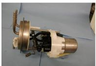
5) Remove the stock fuel pump assembly from the module.
