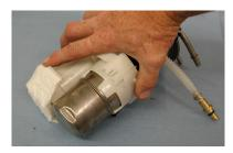
22) Make sure the re-coil spring is positioned in the bucket.
