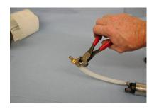
14) Plug the new fuel pump harness wires into the top of the fuel pump.
