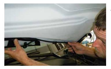
31. Pop the three (3) plastic windshield washer water line retaining clips into place.
