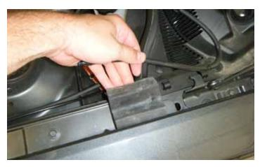
32. Re-connect the windshield washer water line by snapping the line back into the outline line as shown.
