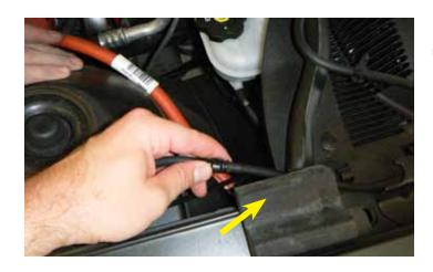
33. Route the windshield washer water line under the foam hood stop indicated.
