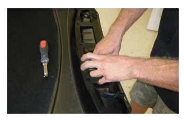
29. Remove the windshield washer water line bracket from the underside of the hood by pulling up from the middle of the bracket.
