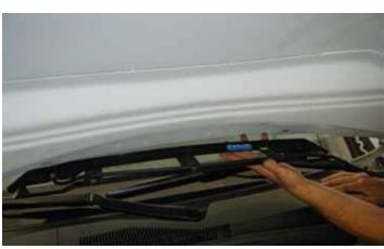
30. Install the windshield washer water line bracket on the underside of the LPE ram air hood as shown. The bracket will snap into place.
