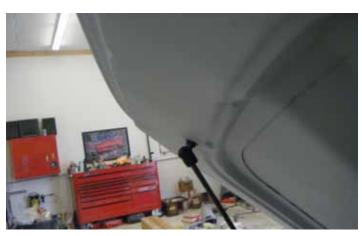
18. Press the prop rod onto the snap fitting joint/fastener until it snaps into place.
