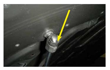
12. Locate the hood prop snap fitting on the underside of the hood. You need to insert a small flat head screwdriver into the slot behind the retaining ring as shown.
