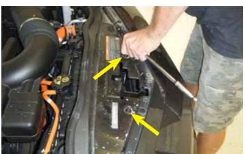
22. Using a Torx-20 socket and ratchet, adjust the front fascia up/down by turning the fascia adjustment bolts clockwise/counterclockwise to line up with the hood.
