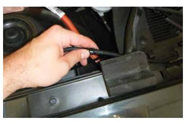
8. Remove the washer fluid line from under the hood stop pad located on the driver side of the engine bay as shown.
