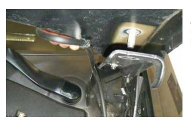
15. While holding the hood in place, completely remove the four (4) nuts securing the hood to the hood mounting brackets. Set the hood aside on a soft clean surface.
