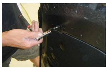
14. Using a 13 mm deep well socket, remove the prop rod snap fitting joint. Be sure to keep the snap fitting joint as it will be re-used.
