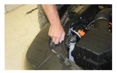
23. Adjust the two (2) rubber hood stops to move the hood up or down depending on which way the adjustment needs to be made. This adjusts the height of the hood when closed.
