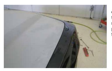
27. Close the hood and check for alignment on the passenger and driver side, as well as the front of the hood relative to the fascia. You may need to repeat steps 11-17 several times to properly align the hood with the fenders and front fascia.
