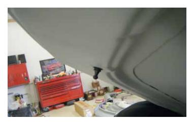
17. Using a 13 mm deep well socket, install the prop rod snap joiny fitting into the ram air hood. Be sure to have an assistant hold the hood up while you install the hood prop rod. Take care to ensure this is tight and secure but be sure to not overtighten.
