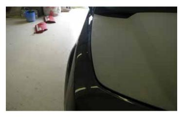
20. Slowly close the hood. Be careful not to damage the LPE hood or fenders. Check the hood lines and make a note of where you need to adjust the hood from the passenger and driver side.
