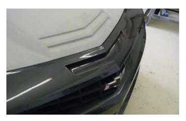
21. Check the front of the hood for any gap and make note of whether the hood needs to move up or down relative to the front fascia.
