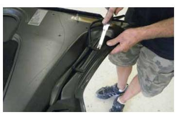
28. Using a pry tool (or equivalent), remove the three (3) windshield washer water line retaining clips from the stock hood.
