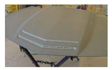
1. Step 4 is only required if you are installing the LPE hood grille inserts for functionality. Installation of the grille inserts requires drilling 6 holes into the upper and lower grilles, three (3) per grille insert.
