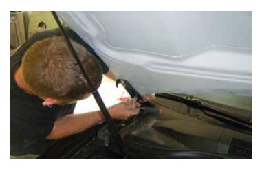
25. Using a 13 mm socket and ratchet, torque the four (4) hood nuts to the hood mounting brackets and adjust as necessary to properly align the hood. Torque these nuts to 18 ft-lbs (25 N-m). The hood bolts can move in any direction so you may need to repeat this process several times in order to properly align the hood.
