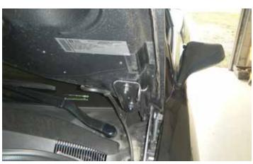
10. The hood is connected by two (2) 13 mm nuts on the driver and passenger side (four nuts total). Loosen the two (2) nuts on the driver side but do not remove them completely.
