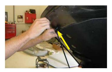
13. While an assistant holds the hood in place, use a small flat head screwdriver (or equivalent) to pry the retaining clip back on the hydraulic prop rod and pull the prop rod away from the hood until it pops out of the snap fitting.
