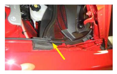
9. Disconnect the windshield washer water line connector by squeezing the connector and pulling the two lines apart.
