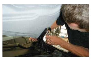
16. With the help of an assistant, mount the LPE ram air hood and start each of the four (4) 13 mm nuts that secure the hood to the hood mounting brackets. Do not tighten the bolts completely.
