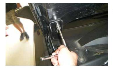
11. Loosen the two (2) nuts on the passenger side but do not remove them completely.
