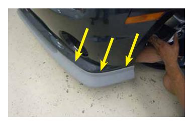
5. This picture illustrates the front chin spoiler installed on the front fascia. The contact points of the chin spoiler shown should be flush with the front fascia.
