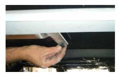
9. Start the driver side 10 mm bolt by hand in the location shown.
