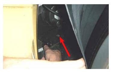
4. You will need to peel back the wheel well lining in order to reach the 10 mm nuts which will need to be tightened evenly. There are six (6), three (3) on each side of the bumper.
