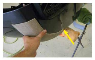
1. Place the passenger side and driver side bolt template into position. The optional installation templates will line up with the curvature of the bottom of the body as indicated.
