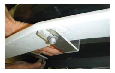
11. Insert the lower support bolt on the front splitter in the slot on the splitter bracket. Using a 10 mm socket and ratchet, torque the two (2) bolts to 62 in-lb (7 N-m) as well as the M6 X 1mm nut with a 16mm washer (PN:MP50)
