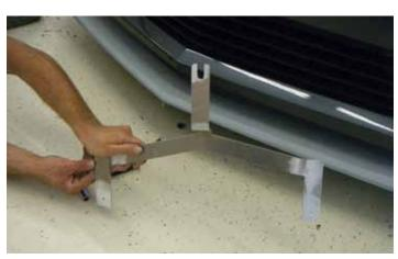
6. This is the front chin spoiler support bracket. This will be mounted under the chin spoiler to give extra support to the front spoiler.
