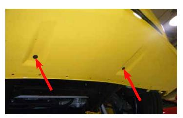
7. The two (2) bolts shown in this illustration are where the two (2) holes on the chin spoiler support bracket are mounted in the next step. Remove these bolts with a 10 mm socket and ratchet.
