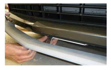
8. Place the chin spoiler support bracket under the middle of the vehicle in the position shown. The two (2) bolt holes spaced 17 inches apart under the front of the Camaro from which you removed the 10 mm bolts is where the spoiler bracket will bolt to the car.
