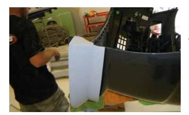
3. Install the chin spoiler using the supplied M6 x 1 mm nuts. There are six (6) mounting bolts built into the chin spoiler that the nuts will install onto.
