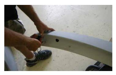
9. There are six (6) of these height adjustment studs. Be sure each height adjustment stud is out far enough that you can fully thread the mounting nuts onto the mounting studs after it is installed on the trunk deck but leave at least 3 (three) turns of thread engagement.
