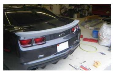
20. If needed, the replacement emblem should be installed at this time. The installation of the LPE rear spoiler is now complete.
