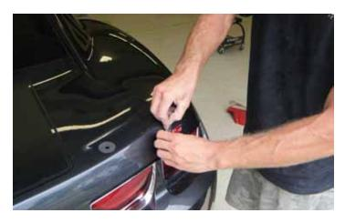
13. If your vehicle has emblems in this area, they will interfere with the installation and must be removed. Using a heat gun and a plastic putty knife (or equivalent), carefully remove the emblem from the trunk deck.
