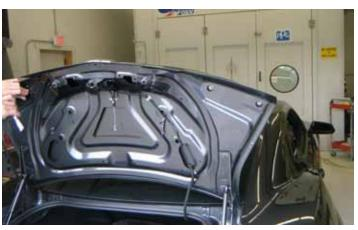
6. Using a 10mm socket and ratchet, remove the six (6) nuts that secure the OEM rear spoiler. The spoiler may fall once all nuts are removed, have someone hold the spoiler in place while the last bolts are completely removed.
