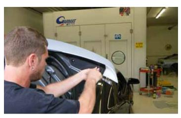
16. Using an allen wrench, adjust the six (6) mounting studs into the spoiler as far in as possible while still maintaining full thread engagement on the OEM M6 X 1mm stainless nuts. Torque these nuts to 53 in-lbs (6 N-m). If full thread engagement is not achieved, use a 3 mm allen wrench to un-thread the studs a bit to ensure full engagement on the nuts.
