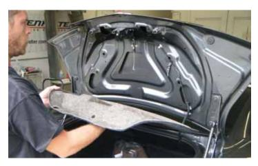
4. Remove the carpet lining. Place the lining somewhere where it will not be damaged.
