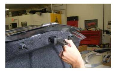
19. Re-install the carpet lining, trunk release lever and the latch guard.
