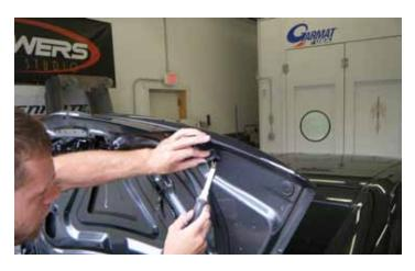
5. Using a pry tool (or equivalent), remove the rubber seal caps on the underside of the trunk as shown. Be careful to not scratch the trunk deck.
