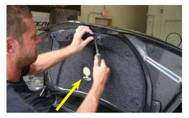
3. Avoid breaking the pop rivets as they will be re-used to secure the trunk deck carpet lining. If you need to replace any of these clips the part number is 11589289. Ensure the trunk release lever is unhooked.
