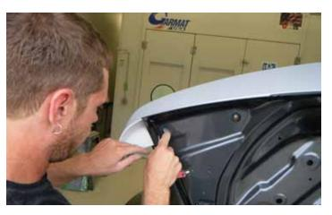
15. Using a 10mm socket and ratchet, install the six (6) OEM M6 X 1mm stanless nuts after applying the loctite supplied in the kit. (PN: 1568 5170)
