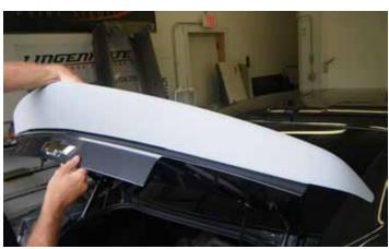
14. Gently set the LPE spoiler in place making sure not to scratch the paint with the mounting studs.
