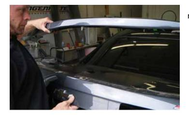
7. Once all of the bolts are removed, carefully remove the OEM spoiler from the trunk.
