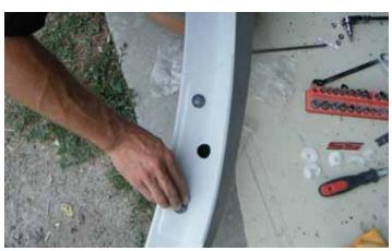
10. Install the six (6) rubber bolt gasket stickers (PN: 20733729) onto the mounting studs.
