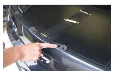
12. Plug the locating hole indicated using the supplied plug/tape.
