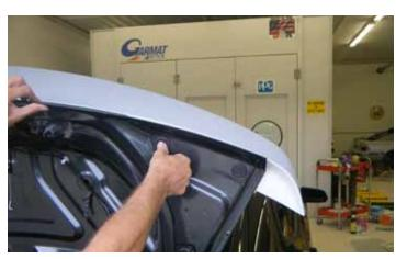
18. Re-install the rubber seals that you removed in step 5 by pushing the center of the seal inward until it snaps into place.
