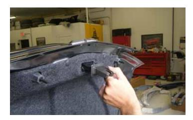
1. Pop the trunk. Remove the trunk latch cover. Use a pry tool (or equivalent) if necessary but be careful to not deform the cover.
