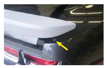
17. The two (2) bumpers that are included in the kit are used to prevent scratching due to overslam on the right and left sides of the quarter panel. Place these bumpers in the position shown. You may place these either on the underside of the spoiler or on the vehicle itself.
