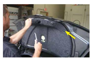
2. Using a pry tool (or equivalent), gently remove the twelve (12) pop rivets that secure the trunk deck carpet lining.
