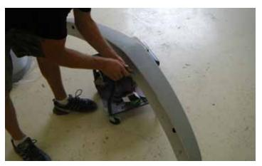
8. Unscrew the height adjustment studs as far as possible on the LPE spoiler.
