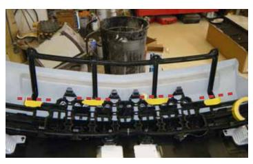
22. Using scotch tape (or equivalent), mark the cutoff points on the bottom of the valance support arms as shown. The dashes illustrate the cutting points.
