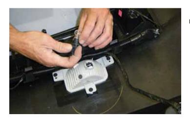
25. Re-install the passenger and driver side reverse lights.
