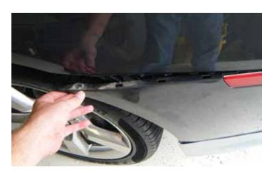
37. The sides of the bumper have clips that line up with clips on the quarter panel.
