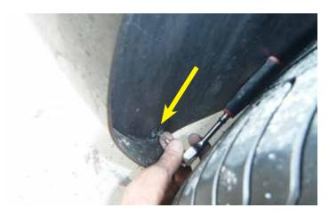
4. Using a Torx 20 socket and ratchet, remove the two (2) bolts inside the wheel wells on the driver and passenger sides of the vehicle.
