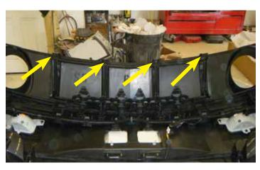
10. Using a 7mm socket and ratchet, remove the four (4) bolts located on the inside of the rear fascia.
