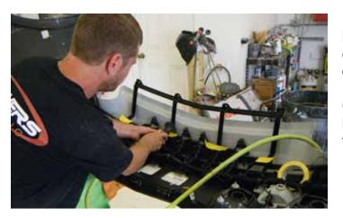
23. Using a cut-off tool (or equivalent), cut the braces at the outermost edge of the tape. This cut is not required to be done while still installed on the bumper.
