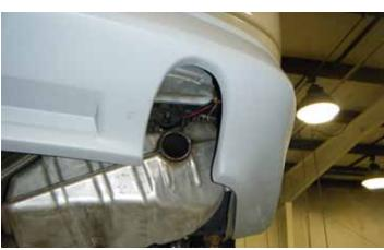
30. Using a hacksaw (or equivalent), cut the exhaust tips off of the mufflers as shown. You will want to get as close to the mufflers as possible.
