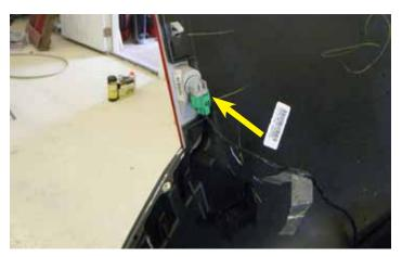
8. Un-install the passenger and driver side turn signal lights.
