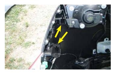
33. The red clips that are illustrated in the next step clip into these slots. These slots are located on the driver and passenger sides of the rear bumper.
