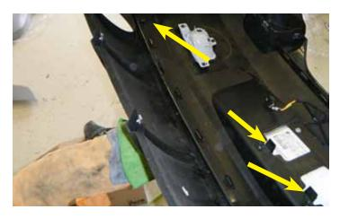
13. Remove the plastic valance energy absorber (already removed in this illustration) by un-clipping the clips that are shown by the arrows. There are four (4) clips total.
