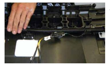
27. Re-connect the wiring harness electrical connector that was removed in step 8.
