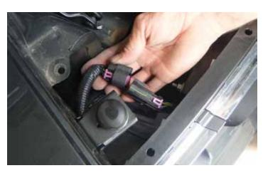
2. Once the cover is removed, disconnect the tail light wiring harness electrical connectors on both sides of the bumper.
