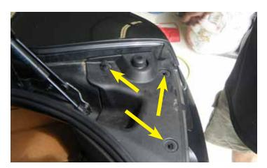
1. Pop the trunk lid. Prepare a clean work surface for when the rear bumper is removed Using a pry tool (or equivalent) remove the pop rivets shown, located above the passenger and driver side tail lights. Make sure not to damage or lose them as they will be used later to re-install this cover.
