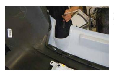
18. Using a 7mm socket and ratchet, install the LPE valance using the holes that were drilled in the previous step. Torque the supplied M6 X 1mm nuts to 89 in-lb (10 N-m).
