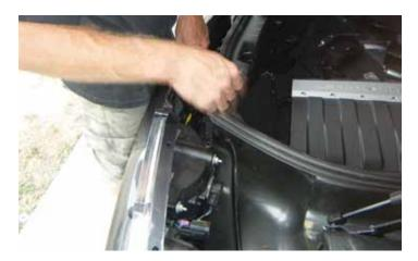
35. Center the bumper and push it onto the red clips until it snaps into place.
