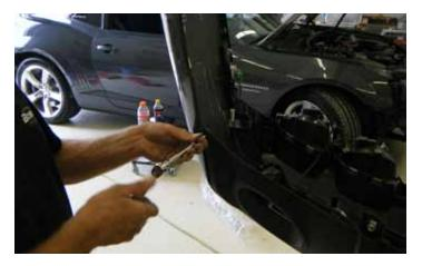
11. Using a 7mm socket and ratchet, remove the two (2) bolts located on the outside edges of the bumper. This illustration shows the location of the bolt on the passenger side.
