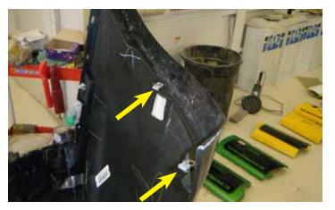
3. This illustration shows the location of the bolts that need to be removed in order to remove the bumper.
