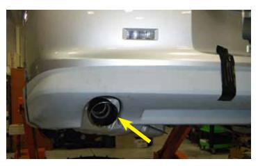
32. Weld the extended exhaust tips to the muffler as illustrated. This is an illustration of how the extended exhaust tip should be set in place in relation to the new rear valance.
