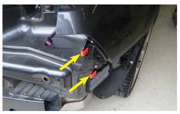
34. Line up the red clips on the driver side and passenger side of the vehicle to the slots illustrated in step 33.
