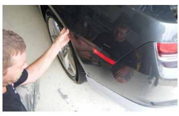
38. Both the driver side and passenger side will snap into place, this will ensure that everything lines up correctly.
