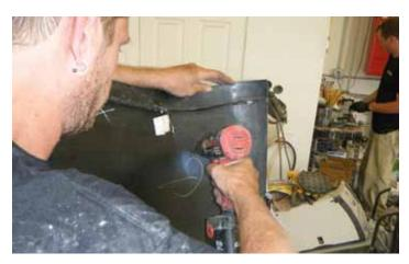
20. Using a 0.25" drill bit and drill, drill out both sides of the bumper that were marked in the previous steps. You will want to drill from the inside of the bumper.
