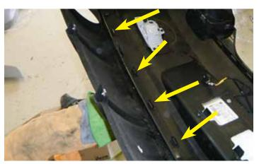
14. Remove the valance from the rear bumper. Be careful not to break the clips. The clips are illustrated by the arrows, but NOTE that not all clips are shown in this picture.
