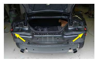
5. This illustration shows the location of the red clips that hold the bumper in place. Be sure not to damage or lose these clips. If you are in need of a replacement clip, the part number is 92223721.
