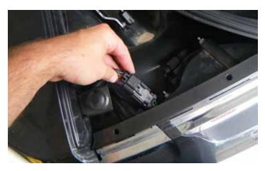
40. Connect the tail light wiring harness electrical connectors on both side of the bumper.
