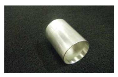
29. This is an illustration of an intermediate exhaust tip extension that will be welded on to the OEM muffler tip. This extension will also work with some aftermarket exhaust systems depending on the diameter of the tubing.
