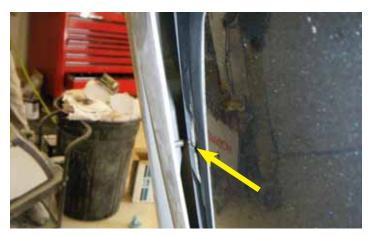
19. Using the M6 X 1mm studs located on the sides of the LPE rear valance, mark the locations on the rear bumper that will be drilled out in the next step.
