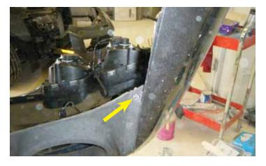
12. Here is an illustration of the other outside bolt that needs to be removed on the driver side of the vehicle.
