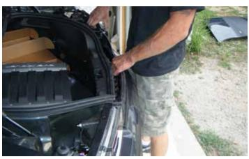
6. Remove the bumper by pulling outward on the driver and passenger side while lifting the bumper away from the vehicle.
