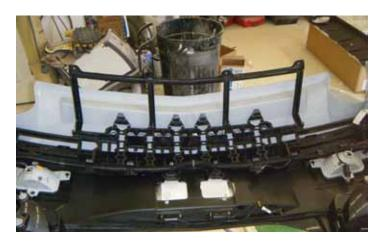
21. Re-install the valance energy absorber that was removed in step 12. The valance energy absorber will be modified in the next step. It will be permanently changed.
