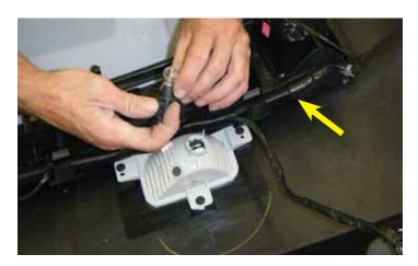
9. Remove the reverse light bulbs as well as the rear bumper wiring harness from the rear bumper.
