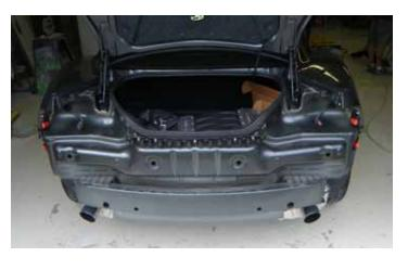
28. The LPE valance sits farther back from the OEM GM valance. Because of this the exhaust tips on the stock OEM exhaust and some aftermarket exhausts will need to be relocated. To do this you will need to cut the exhaust tips and weld the supplied extensions in place. The supplied extensions are designed to work with the stock exhaust and may work with some aftermarket exhausts. Custom extensions may be needed for some applications.
