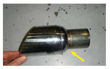
31. Weld the extensions to the OEM exhaust tips as shown in this illustration. Take care to make sure the extensions are concentric with the exhaust tips.
