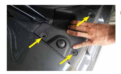
41. Place the tail light wiring covers and reinstall the pop rivets.
