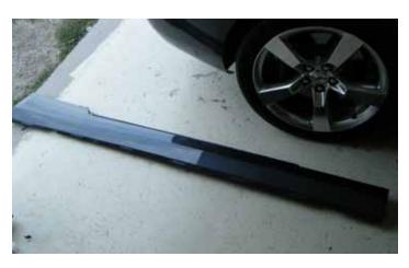
8. With the retaining clips removed, set the OEM rockers safely aside so they do not get damaged.
