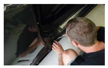
5. Continue prying the rockers off of the vehicle while gently pulling the rockers away from the vehicle. Be careful not to damage the retaining clips, they will be used in the installation of the LPE rockers. If you need replacement retaining clips, you can find the part number in the "Optional Items" parts list (11610495).
