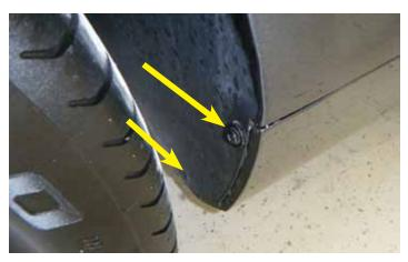
2. Using a Torx 20 socket and ratchet, remove the bolts indicated.
