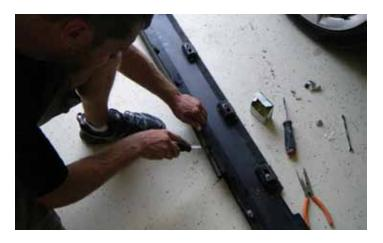
15. Using a pry tool (or equivalent), carefully remove the weather stripping from the OEM rocker by prying out the tree style rivets that hold the weather stripping in place. This weather stripping will be used on the LPE rocker. Inspect the weather stripping for damage or wear. If you need to replace your weather stripping, the GM part number is 92238467.
