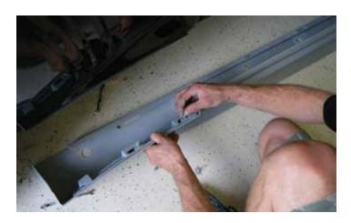
9. Install the retaining clips removed in step 7 into the LPE rocker by inserting them and sliding them into place as shown. Be sure not to damage the retaining clips.
