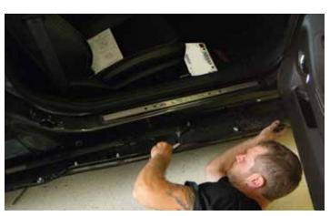
6. Remove the rockers from vehicle. Be careful when removing the rockers, they can easily be damaged if forced during the removal process.
