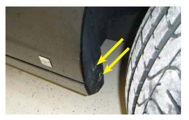
3. Locate the wheel liner securing bolts on the passenger front side of the vehicle and, using a Torx 20 socket and ratchet, remove the bolts.
