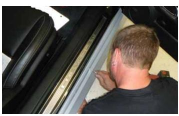
14. Install the thirteen (13) supplied rocker bolts (PN: AV13026) into each hole on the rocker, these will be installed into the grille nuts. Be sure these bolts are tight and secure but do not overtighten.
