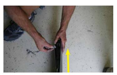
7. Remove the retaining clips from the rockers by sliding them toward the front of the rocker, be sure not to break any of the clips as they will be re-used on the LPE rocker. If any are damaged the replacement part number is 11610495.
