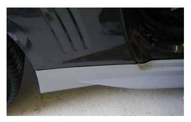
13. Place the rocker into position on the vehicle. The retaining clips will clip into place. You may need to adjust the retaining clips slightly from side to side to ensure the rocker is lined up correctly.
