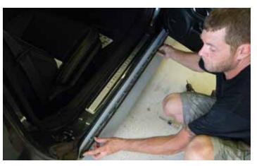
16. Install the weather stripping onto the LPE rocker by pushing each tree rivet into the holes as shown.
