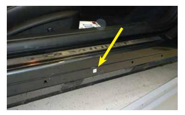
11. Insert the supplied white size 10 grille nuts (PN: AV13933) into the rocker panel on the vehicle. Be sure the grille nuts are securely inserted into each spot.
