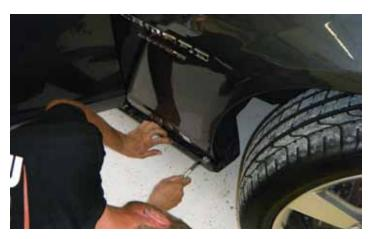
4. Using a pry tool (or equivalent) start at the front of the vehicle and pry the stock side rockers off of the vehicle.
