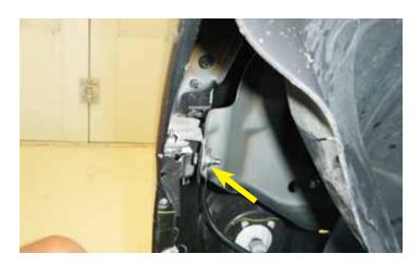
29. Using a 10 mm socket and ratchet, reinstall the nut that is located in passenger and driver side wheel wells. Torque this bolt to 62 in-lbs (7 N-m).
