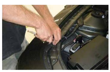
2. Open the hood to the vehicle. Using a 10 mm socket and ratchet, remove the two (2) bolts shown on the passenger side front of the front fascia. Save these bolts as they will be used in re-assembly.
