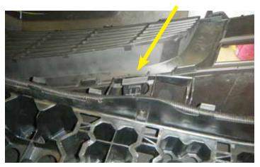
15. Un-clip the clip on the passenger side of the fascia illustrated by bending the larger tab (indicated by the arrow) away from the smaller tab below it and pulling upward.
