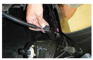
12. Disconnect the front fascia wiring harness electrical connector and remove the front fascia from the vehicle.
