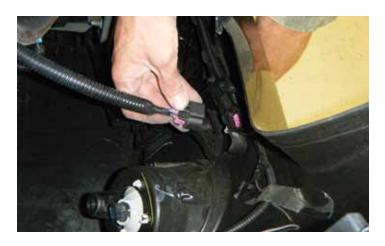
25. Re-connect the wiring harness electrical connector on the inside of the front fascia.
