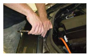
3. The second bolt is located directly in front of the fuse panel on the passenger side.
