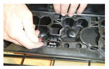
19. There are sixteen (16) retaining tabs that hold the grille in place. Using a small flat head screwdriver, remove the grille from the fascia by popping each of the tabs out of the retainers on the grille while pulling the grille upward.
