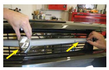
24. This illustration shows the placement of the LPE shield and emblem that are to be placed on the grille insert after it has been painted. These locations are the same for the carbon fiber insert as well.
