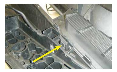
16. Un-clip the clip on the driver side illustrated by bending the larger tab (indicated by the arrow) away from the smaller tab below it and pulling upward. Remove the fascia support webbing.
