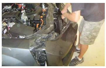
26. Place the bumper onto the front of the vehicle. Take care to not scratch the bumper or quarter panels.
