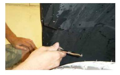
7. Remove the three (3) scrivets, as illustrated, on the driver side of the vehicle.
