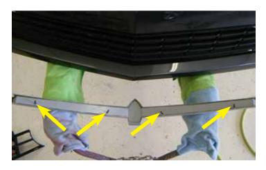
21. The LPE front fascia grille insert should be installed next. Notice the four (4) studs on the back of the insert, these will secure behind the grille with the supplied four (4) nuts and special tabbed washers.
