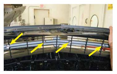
23. Using the supplied tab washers and M6 X 1 mm nuts, secure the LPE grille insert by tightening them down with a 10 mm socket and ratchet.
