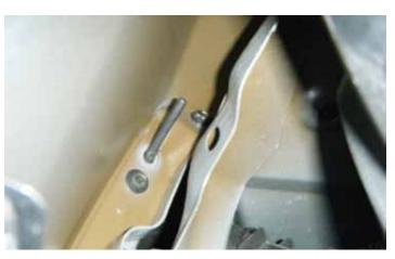
28. Using a 10 mm socket, re-install the two (2) bolts located inside the driver and passenger side wheel wells. Torque these bolts to 62 in-lbs (7 N-m)
