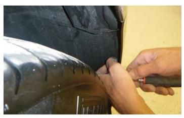
6. Using a Torx 20 socket or driver, remove the three (3) scrivets on the passenger side of the vehicle.
