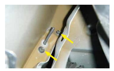
9. Using a 10 mm socket and ratchet, remove the two (2) bolts indicated. These bolts are located directly above the bolt removed in step 7. Step 7-9 are to be repeated for the passenger side.
