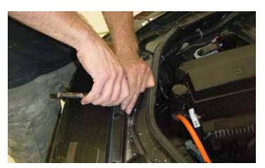
31. Using a 10 mm socket and ratchet, install the six (6) bolts for the top of the bumper supports removed in steps 1-3. Torque these bolts to 62 in-lbs (7 N-m).
