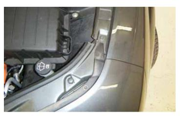
4. Remove the two (2) bolts on the driver side. These bolts are mirrored in the same position as the passenger side.
