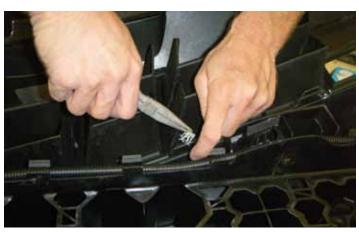
18. Remove the grille retaining clip on the passenger side of the front fascia located on the inside of the front fascia as shown.
