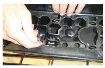
14. Using a small flat head screwdriver, un-clip the clip on the fascia support webbing located in the middle of the inside of the front fascia.
