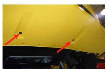
10. Using a 10 mm socket and ratchet, remove the two (2) lower support bolts under the front fascia of the vehicle.
