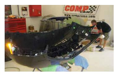
13. With the help of an assistant, place the front fascia on a clean work surface as shown. You will need access to both the inside and outside of the fascia during this part of the installation.
