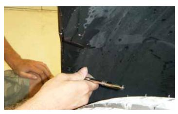
30. Re-install the three (3) scrivets located in the passenger and driver side wheel wells. Torque these scrivets to 27 in-lbs (3 N-m).
