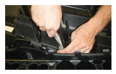
17. Using a pair of needle nose pliers, remove the grille retaining clip on the driver side of the front fascia located on the inside of the front fascia as shown.
