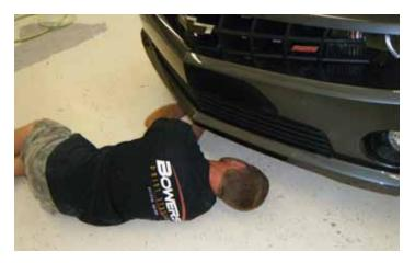
27. Using a 10 mm socket and ratchet, reinstall the two (2) lower support bolts and torque to 62 in-lbs (7 N-m).
