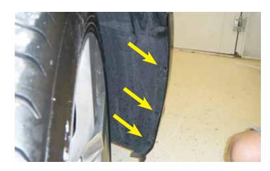
5. There are three scrivets on the passenger side of the front wheel well liner.
