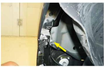
8. Peel back the front wheel well liner and using a 10 mm socket and ratchet, remove the bolt shown. The other two (2) bolts are located directly up from this bolt.
