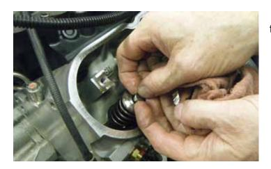
13. If applicable, re-install the lash caps onto the valve tips.
