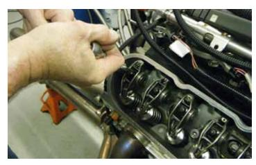
14. Re-install the rockers onto the engine using your engine's recommended torque setting.
