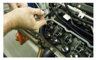
3. Remove the rockers from the valves and valve springs.
