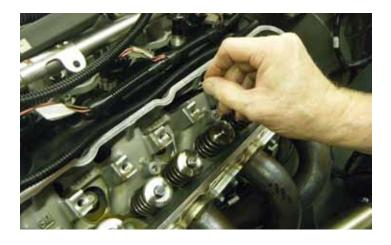
12. Re-install the pushrods into the motor.
