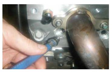
6. Install the cylinder leak tester into the cylinder and fill the cylinder with air.
