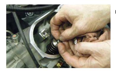
5. On LS7 and LS9 applications, remove the lash caps from the intake valves.
