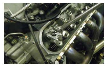
7. Using one of the production rocker arm bolts, install the valve spring compressor into the rocker arm support.
