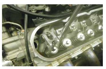
8. Using a 3/8" ratchet, insert the ratchet into the square hole located on the end of the compressor tool. Compress the spring and remove the valve spring locks (keepers) and retainers. A small screwdriver with a magnet or other magnetic retrieval tool may help.
