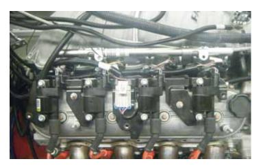
1. Remove the engine covers, coil packs, fuel lines (if necessary to get to the valve covers), and anything else necessary to remove the valve covers from the vehicle. Remove the spark plugs so you can pressurize the cylinders with air.
