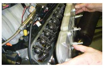
2. Remove the valve covers from the vehicle. Inspect the valve cover gasket for damage or wear and replace if necessary.
