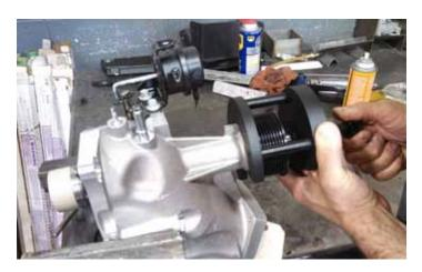
4. Place the pulley removal tool over the back of the supercharger pulley and hand tighten the bolt so that the bolt is pressing against the center of the shaft.
