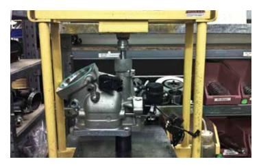
13. Place the hub or pulley onto the shaft and carefully press the part onto the shaft.
