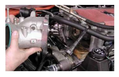
You must remove the supercharger front cover from the supercharger assembly to change the pulley. This is because you must support the shaft when pressing the new pulley on or you will cause the shaft to move in the cover housing and it will need to be rebuilt/serviced.
