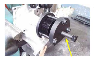
5. Make sure the threads on the pulley removal tool bolt have anti-seize on them. Failure to do so will cause the bolt to get hot and seize in the tool, potentially destroying the tool.
