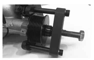
3. Unscrew the primary bolt from the pulley removal tool until the tip of the bolt is just sticking past the inside of the tool.
