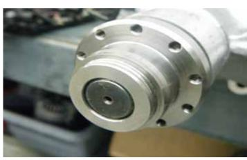
14. The leading edge of the pulley or hub should be flush with the end of the jackshaft, as shown in the image to the left. At this time you may want to also pin the pulley or hub on the shaft. Follow the instructions for doing this found in the LPE pulley instructions.
