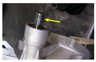
12. Apply press lube to the supercharger shaft.
