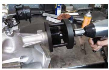
6. Using a ratchet or an impact gun and a 24 mm socket (or 15/16"), tighten the bolt.
