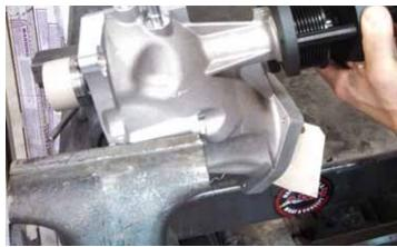
2. Secure the front cover in a vise, being careful not to damage the aluminum casting.
