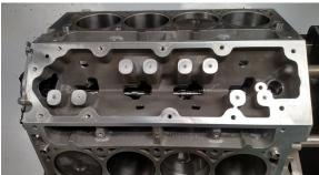
3. Plug one of the 8 holes using the rivet tool.
