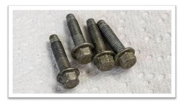
7. Use a lubricant to lube the preinstalled orings on the 4 DOD delete plugs. Press all 4 plugs into actuators sockets in the block.
