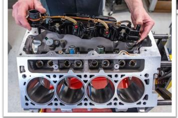
5. Use an 8 mm socket to remove 4 bolts holding DOD actuators to the block.
