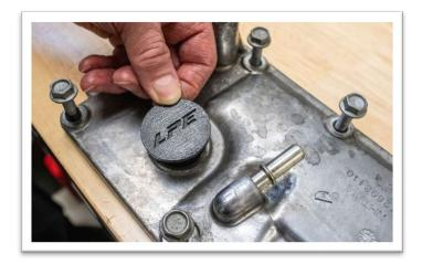
14. Use the provided C clip to secure the valley cover plug to the back side of the valley cover.
