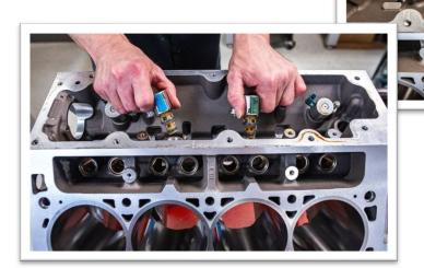
6. Remove stock bolts from OEM actuators for reuse with the C8 Corvette DOD Delete Kit.
