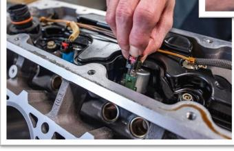
4. Use a 10 mm socket to remove 4 bolts holding the black plastic harness body to the engine block. Remove plastic housing from the block.
