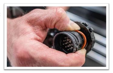
12. Install the OEM oring onto the new DOD delete the valley cover plug.
