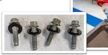
9. Install all 4 fasteners into the block to secure the plugs. Torque to 89 lb-in.
