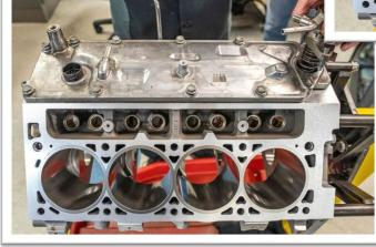
2. Use a 13 mm socket to remove 9 remaining bolts holding the valley cover onto the engine block. Remove valley cover.
