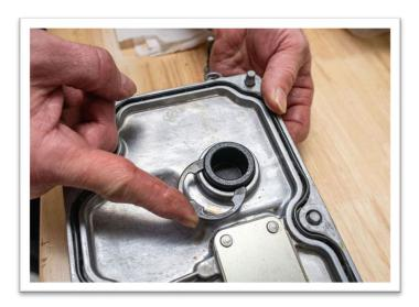
15. Reinstall the valley cover to the engine block and torque 9 bolts to 25 Nm (18 lb-ft) using the provided torque sequence.
