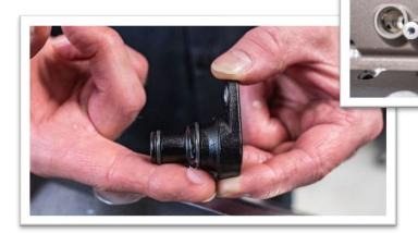
8. Pre-assemble the 4 provided washers onto OEM bolts to hold down DOD delete plugs. Put Blue Loctite onto all 4 fasteners threads.
