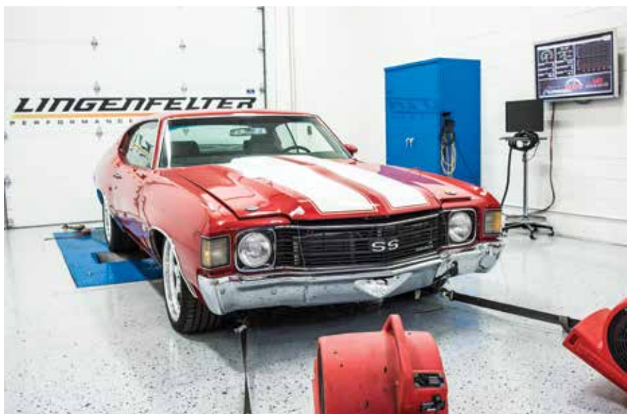
TEST TRACK A 1972 Chevrolet Chevelle is tested for horsepower and torque on a computerized chassis dynamometer. The system will calibrate the different mechanical, fuel, and electronic systems on the vehicle to get the best combination of power and drivability.
