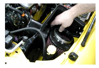
**Step 25** - Install the filter as shown. Make sure the filter is sealed on the air tube with the metal tube fully inserted into the rubber air filter neck. Tighten the clamp.
