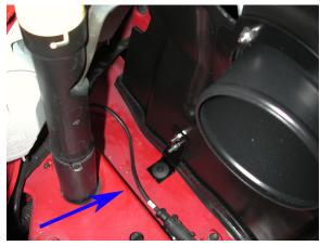
**Step 19** - The Torx head will push into the grommet on the inside of the fenderwell.
