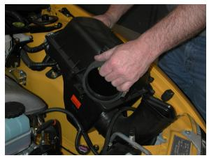
**Step 6 -** In the void where the airbox was, you will see a fastener with a T-30 Torx head, remove this fastener. This will serve as a mounting stud for the air box in a later step.
