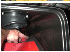
Step 23 - If you had to remove the perforated section of the airbox, make sure the AC line is on the engine side of the airbox except for the small 180 degree section that rests under the seal.
