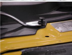
**Step 3 -** Loosen the metal hose clamp that attaches the air tube to the throttle body and remove the stock air tube from the throttle body.
