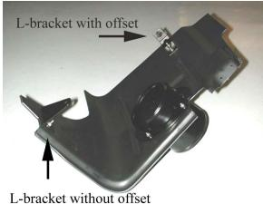
**Step 11 -** Using the supplied M6 flange nut, install the factory Torx head stud (removed in an earlier step) onto the "L" bracket as shown.
