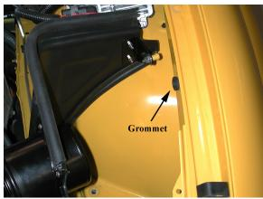
**Step 18** - Make sure this harness routes to the inside of the airbox as shown.
