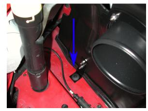
**Step 21** - Using the holes in the top of the air box, ziptie to the aluminum AC tube, around the bottom side of the service port (see picture). The tie should go through one hole, around the AC tube, just above the sensor, and through the 2nd hole. Tighten securely and trim the end of the zip-tie.
