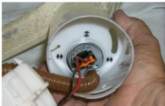
Sliding the lid up the fuel line reveals the fuel pump connections. Remove the electrical connector by squeezing and pulling it out.
