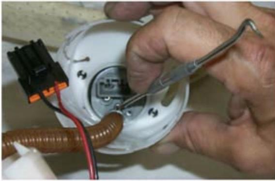
Remove the fuel line connection by carefully spreading the "loop" in the clamp. Do this by using a small tool such as a scribe or small screwdriver and some patience. Take care not to damage the fuel line itself, as it must be reused on the new pump. The clamp will be replaced.
