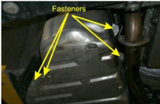
Remove the driver's side rear wheel to gain better access to the fuel pump assembly. Using a ratchet, 10 and 13 mm sockets, remove the two fasteners that retain the end cap on the fuel tank panels.
