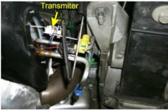
Remove the six bolts that secure the access panel with a ratchet and a 7 mm or 10 mm socket. Pull the access cover and pump assembly out of the tank four to six inches and stop. Note the white plastic fuel level transmitter mounted near the top of the access panel and its thin, metal float arm going back into the tank. Carefully move the float arm through its full range of motion and make note of how far it moves.
