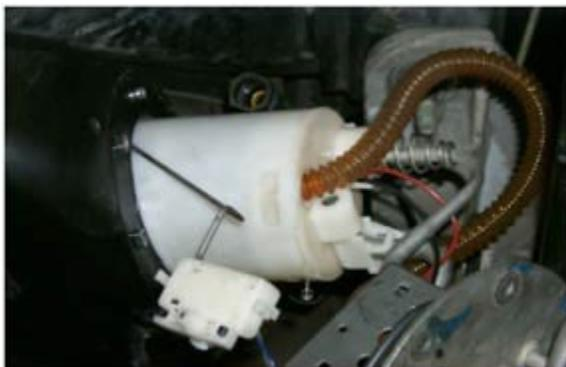
With the fuel level transmitter loose, reach into the opening and pull out the loop of orange plastic fuel line, this will ease removal of the pump assembly.
