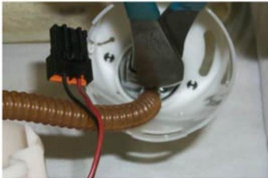
Install the fuel line on the new pump by sliding the new clamp (taped to the can previously) over the end of the fuel line. Slide the fuel line on the nipple of the pump and crimp the loop tightly.
