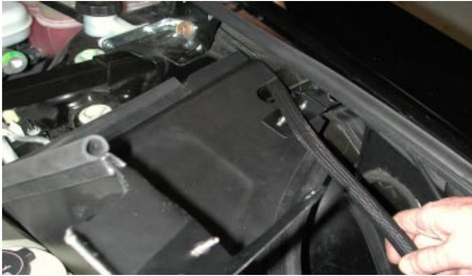
**Step 9. Mounting the rear of the air filter heat shield**
