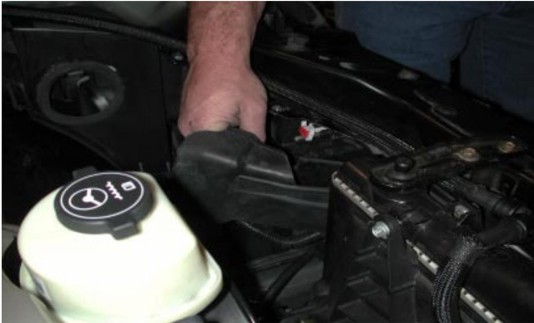
Step 5. Remove plastic rivet
