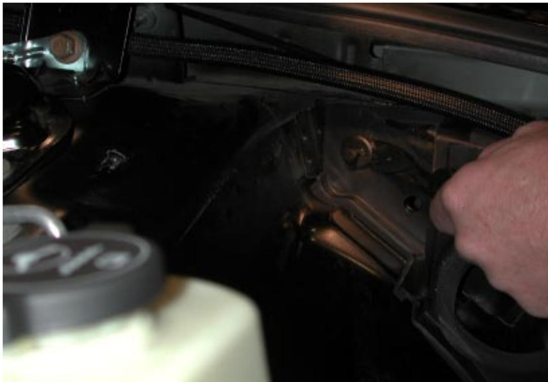
Step 6. Intallation of air filter heat shield mouting brackets.
