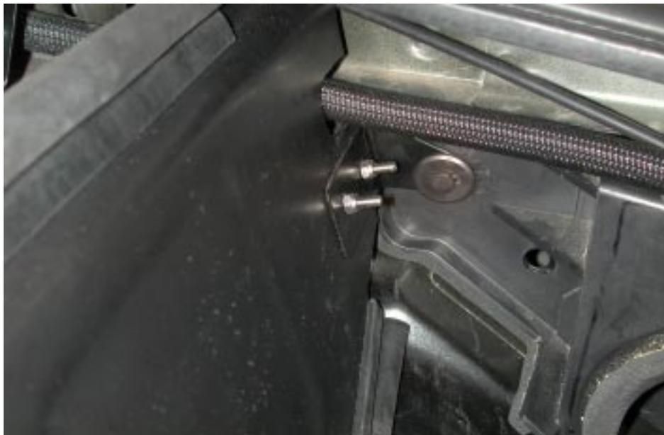
Step 10. Mounting the front of the air filter heat shield
